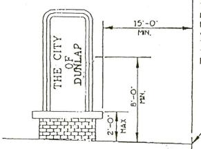
IF ANY PORTION OF A SIGN OTHER THAN THE POLES ON WHICH IT IS MOUNTED. IS MORE THAN 2'-0' OR LESS THAN 8'-0' ABOVE THE GROUND, THEN THE FRONT EDGE OF THE SIGN CAN BE NO LESS THAN 15'-0' FROM THE EDGE OF THE RIGHT-OF-WAY/FRONT PROPERTY LINE.
