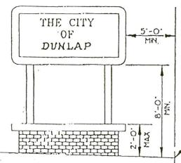
IF NO PORTION OF A SIGN, OTHER THAN THE POLES ON WHICH IT IS MOUNTED. IS MORE THAN 2'-0' OR LESS THAN 8'-0' ABOVE THE GROUND. THEN THE FRONT EDGE OF THE SIGN CAN BE NO LESS THAN 5'-0' FROM THE EDGE OF THE RICHT-OF-WAY/FRONT PROPERTY LINE.
